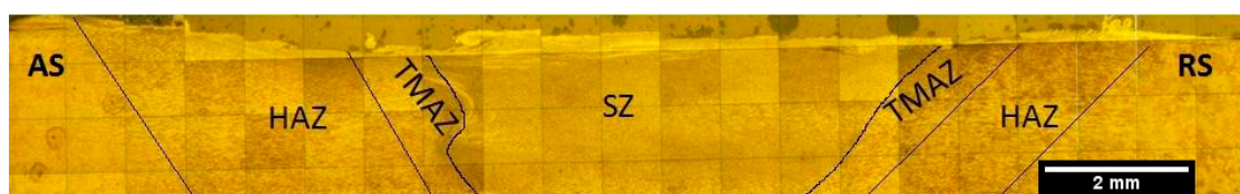
Figure 3. Friction stir welding micro-structural zones.
