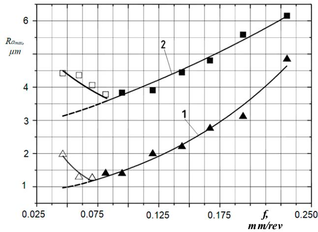
**Figure 2.** Dependence of the sample mean roughness parameter  $\bar{R}_a$  on the feed rate  $f$  for Fe-C alloys: 1—steel 45; 2—cast iron KCh 30-6.
