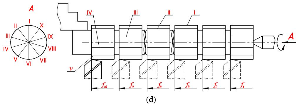
**Figure 1.** Test specimen and schemes of technological semi-rough and finish junctions: **a**—drawing of the test specimen; **b**—general view of the test specimen; **c**—scheme for the implementation of the semi-rough pass; **d**—scheme of finish pass and placement of tracks for measuring parameter  $R_a$ .
