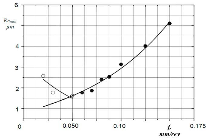
**Figure 3.** Dependence of the sample mean roughness parameter  $\bar{R}_a$  on the feed rate  $f$  for steel 30 KhGSA.
