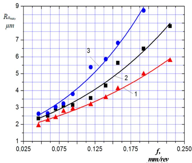
**Figure 4.** Dependence of the sample mean roughness parameter  $\bar{R}_a$  on the feed rate  $f$  for non-ferrous alloys: 1—silumin AL4  $R_{a_{max}} = 1.594 \cdot (1 + f)^{6.321}$ ; 2—duralumin D16T  $R_{a_{max}} = 1.673 \cdot (1 + f)^{7.553}$ ; 3—brass LS63-3  $R_{a_{max}} = 1.655 \cdot (1 + f)^{9.56}$ .
