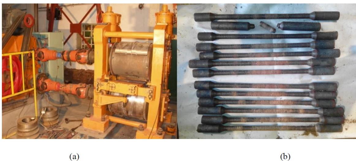
Figure 13. The experiment of the CWR Ti-6Al-4V blade (a) H500 mill; (b) The samples of rolled.
