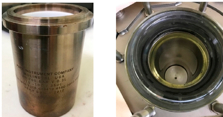
Figure 4. Parr Autoclave with maximum pressure of 200 bar and maximum temperature of 250 °C.
