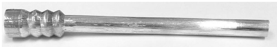
Figure 4. AA6082 billet processed by interrupted gradation extrusion.
