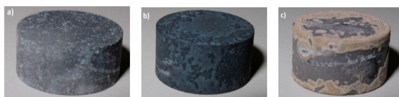
Figure 1. Photographs of the coatings obtained on Ti-15Mo in the electrolytes of series 1, 3, 4 (a); 2, 5 (b), and 6–8 (c).
