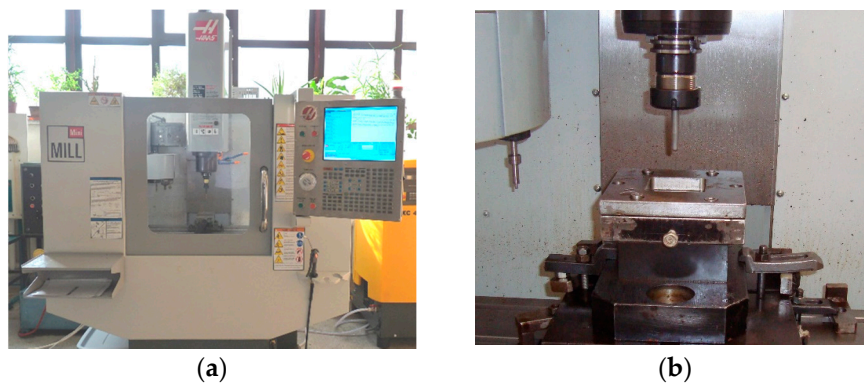
Figure 4. Technological equipment: (a) Haas MiniMill computer numerically controlled (CNC) machining center; (b) Forming equipment (active die and retaining plate).
