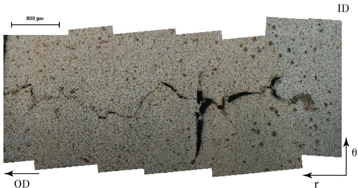
Figure 9. SOHIC at location 500.
