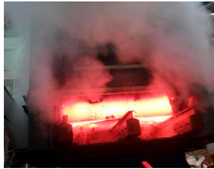
Figure 7. Slab cooling process.
