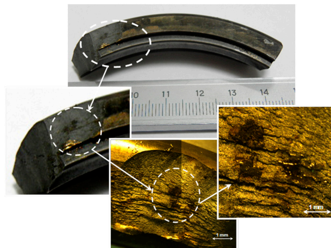
Figure 5. Stereoscopic images of a fragment of the failed outer ring, exhibiting signs of oxidation on the fracture surface.
