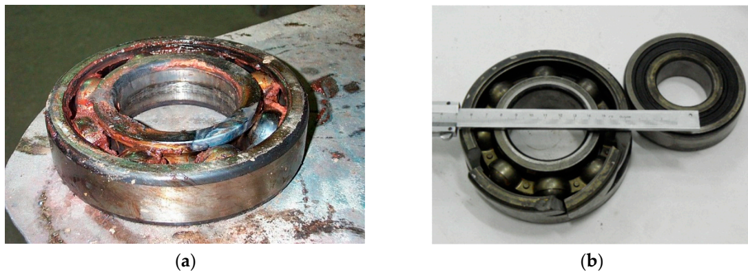
Figure 3. Rolling bearing as-received (a) and after the removal of organic residuals (b).
