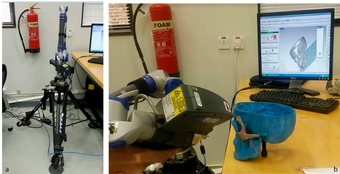
Figure 14. 3D measurement (a) Faro platinum arm with scanner; (b) scanning of the skull model fixed with titanium zygomatic implant.
