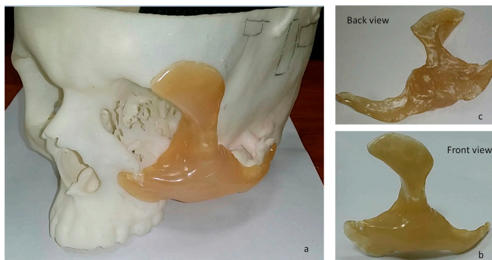
Figure 3. (a) Fused deposition Modeling fabricated skull model with the attached silicone implant; (b) silicone implant front view; and (c) silicone implant back view.
