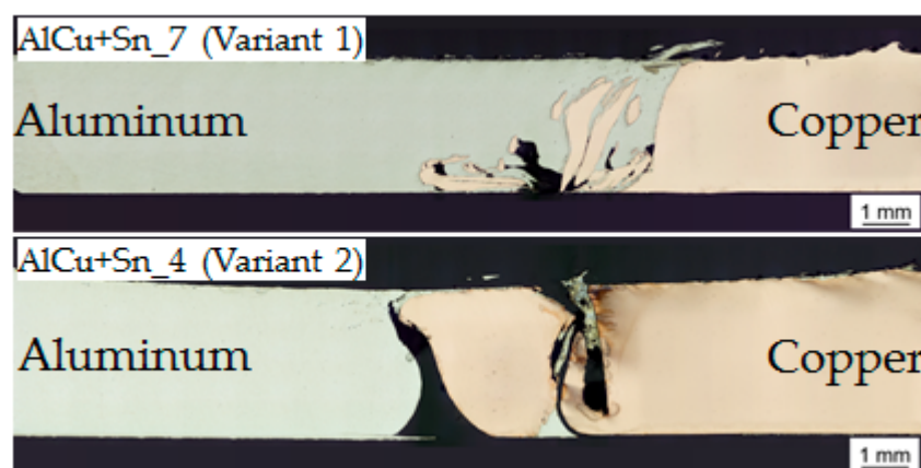
Figure 7. Cross-sectional macrostructures for parameter combinations AlCu+Sn_7 (variant 1) and AlCu+Sn_4 (variant 2).
