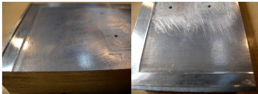
Figure 15. Example of damaged surface due to the use of aggressive parameters.
