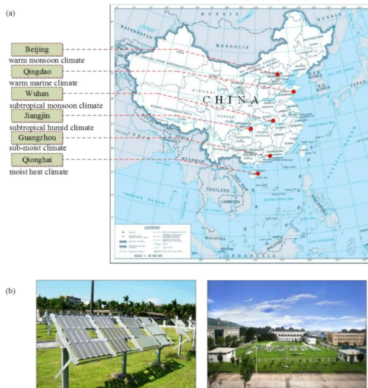
**Figure 1.** (a) The geographical distribution and climate types of 6 test stations; (b) the on-site pictures of exposure test.
