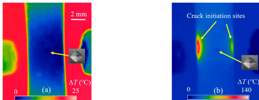
Figure 7. The temperature distribution of the specimen surface obtained by thermography in a 20% CW 316L specimen (indent depth is 45  $\mu\text{m}$ ) tested at 380 MPa, which failed at  $2.75 \times 10^6$  cycles. (a) Before fatigue test; (b) just before fatigue failure. Note:  $\Delta T$  is defined as the specimen temperature changes with respect to minimum temperature at the initial state, as well as in Figure 8.
