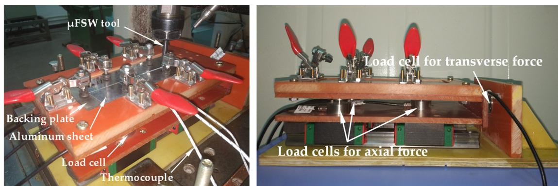
**Figure 2.** The fixture for ultra-thin sheets welding.
