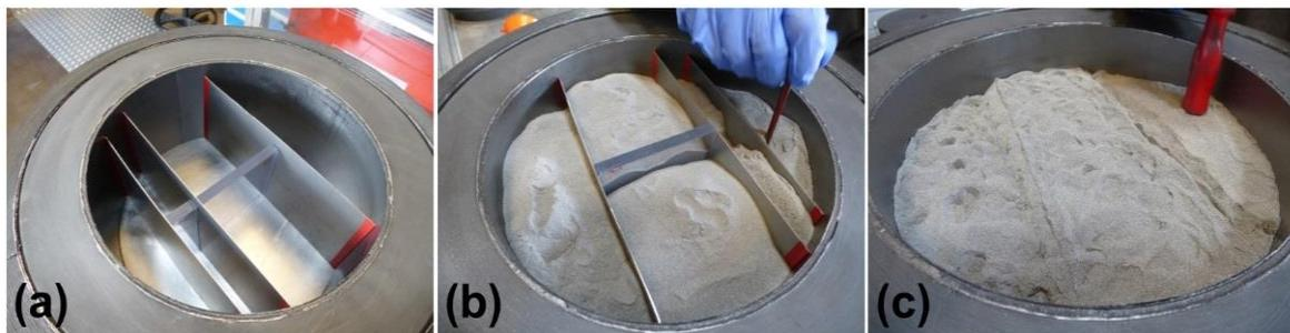
**Figure 3.** Photographs of the large-scale manual powder layup at Kennametal Ltd. UK, showing; (a) titanium sheet and Perspex dividers in the 250 mm diameter mould; (b) dissimilar powders filled in the separate sections with agitation of powder using a brush; and (c) flattening of powder after the dividers have been removed.
