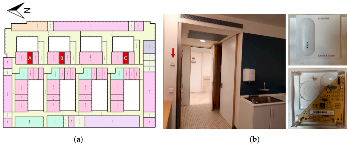
Figure 1. The last floor of the building, selected for the study. (a) Rooms location on the plan from the model view; (b) indoor temperature sensor type and location in the rooms.
