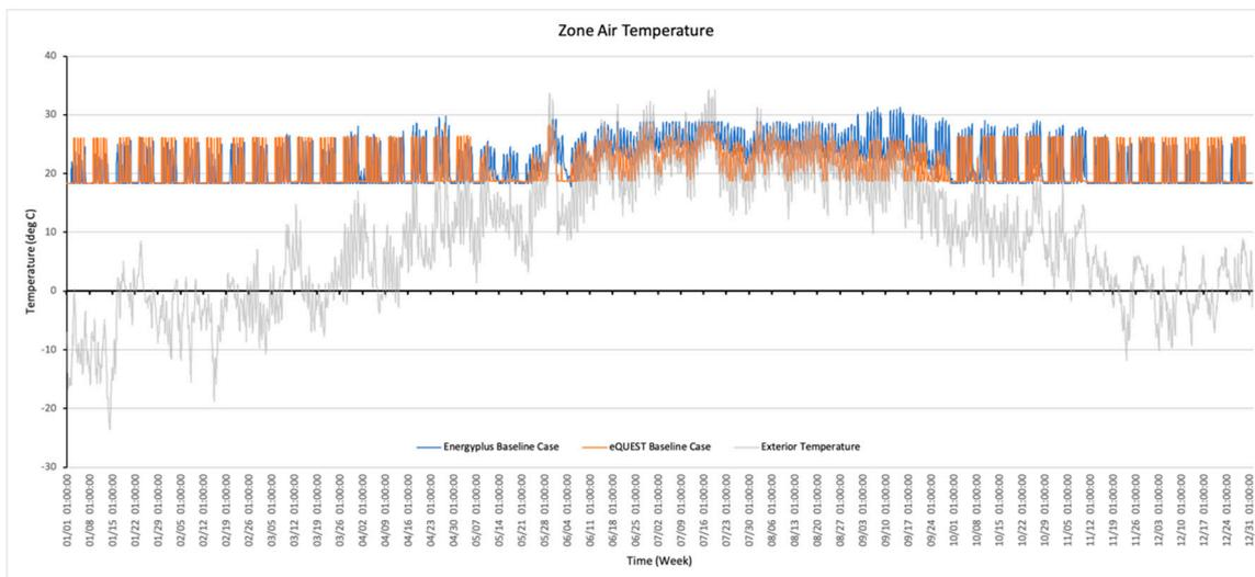
Figure 5. Simulated annual temperature profile from eQUEST and EnergyPlus showing overheating.
