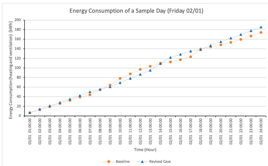
**Figure 13.** Cumulative Energy Consumption (Mechanical Ventilation and Heating inclusive) of a day, comparison between baseline and revised case.
