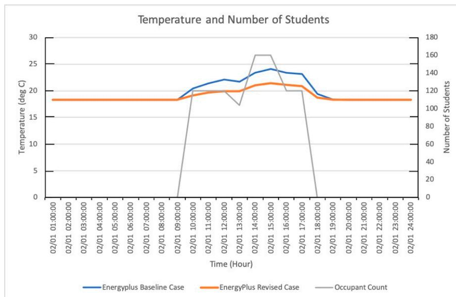
Figure 11. EnergyPlus temperature results of a day, showing a reduction in indoor air temperature.
