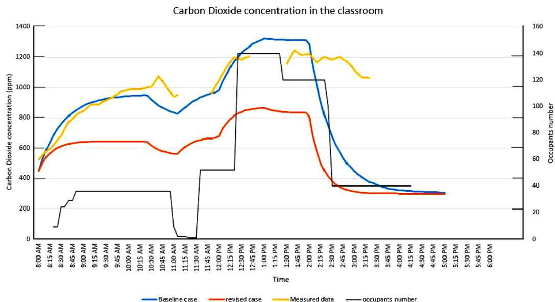
**Figure 8.** Carbon dioxide concentration compared between measured and simulated model. Note that the measured data is segments due to the disruption of the equipment; however, the concentration increase can still be observed.
