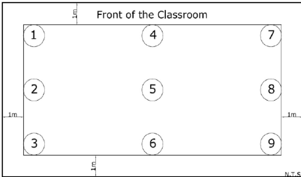
Figure A1. Plan Showing Dataloggers Placement Distribution Across the Classroom.
