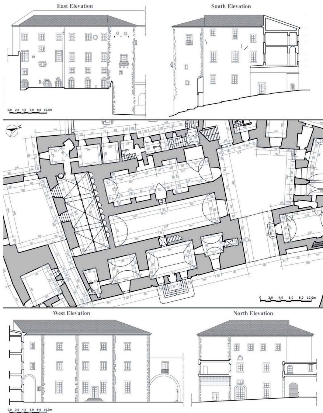
Figure 6. Geometric survey of the ground floor and the elevations of the central part of the Castle of Melfi (PZ), Italy.
