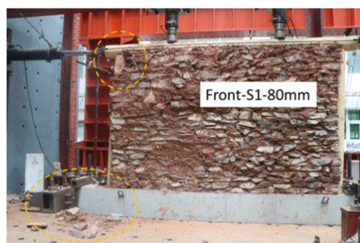
Figure 19. Displacement loading of 80 mm (drift 3.04%) for S1.
