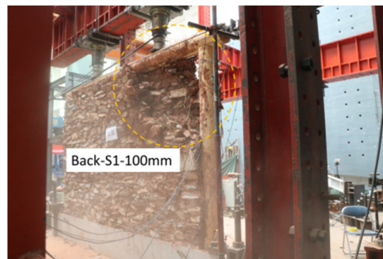
Figure 20. Displacement loading of 100 mm (drift 3.80%) for S1.
