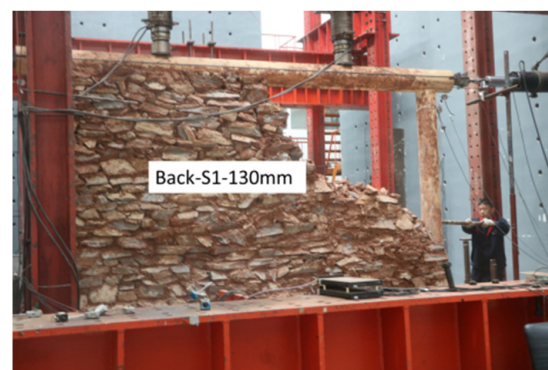
Figure 22. Displacement loading of 130 mm (drift 4.94%) for S1.
