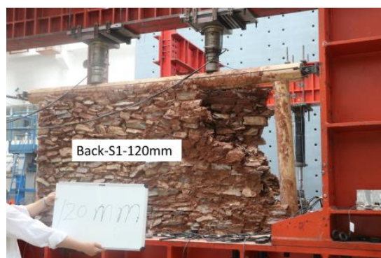
Figure 21. Displacement loading of 120 mm (drift 4.56%) for S1.
