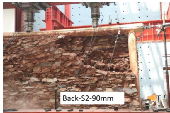
Figure 24. Displacement loading of 90 mm (drift 3.42%) for S2.
