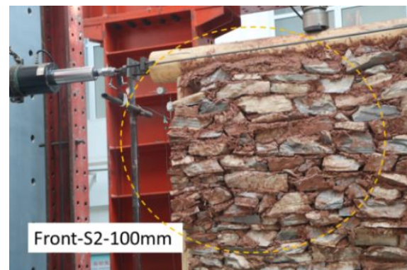
Figure 25. Displacement loading of 100 mm (drift 3.80%) for S2.
