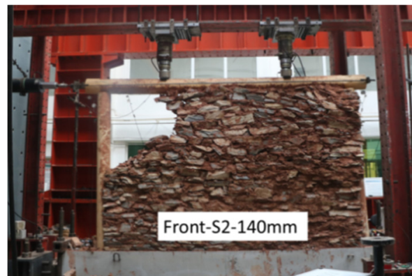
Figure 26. Displacement loading of 140 mm (drift 5.32%) for S2.
