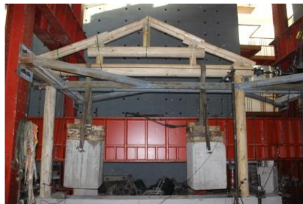
Figure 32. Loading test of the wood frame.
