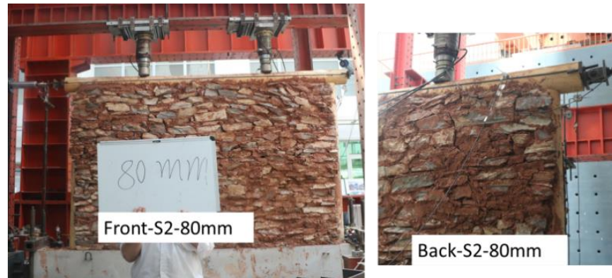
Figure 23. Displacement loading of 80 mm (drift 3.04%) for S2.
