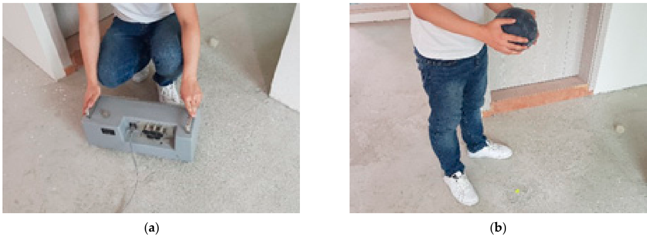
Figure 8. Standard impact sources: (a) tapping machine and (b) rubber ball.
