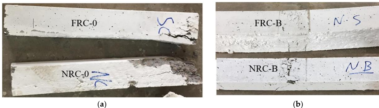
Figure 7. Failure mode of NRC and FRC (a) columns and (b) beams.
