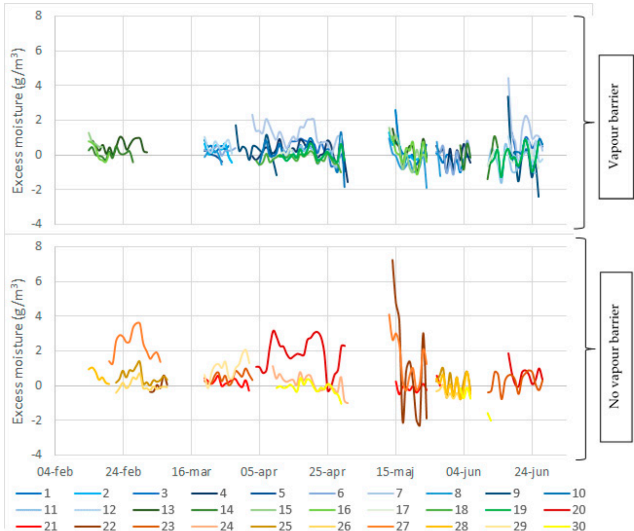
Figure 10. Daily average of excess moisture in the attics. Note that some measurements from house 22 exhibit excess moisture up to 16 \text{ g/m}^3 in single measurements. Top: houses with vapour barriers (1–19), bottom: houses without vapour barriers (20–30).
