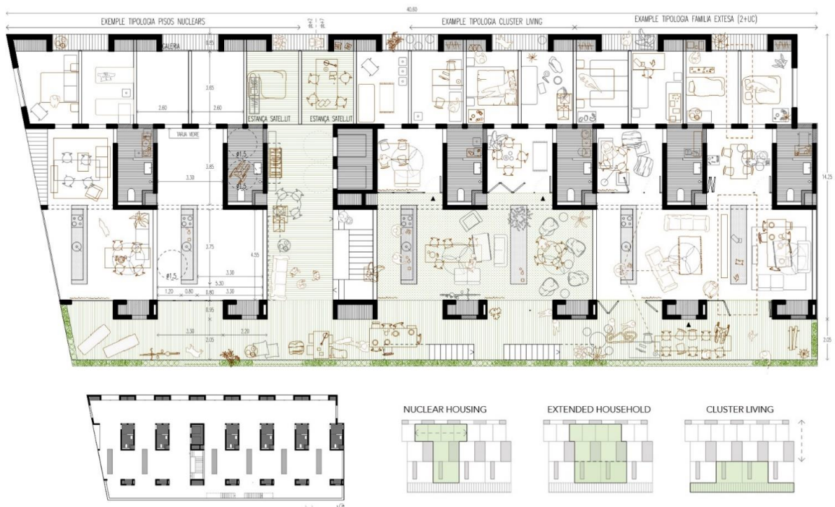
Figure 10. La Quinta Força by Llindarquitectura and Avilla-Royo. Top: plan. Below left: the building is presented without boundaries between dwellings as an open plan to be defined by the cooperative. Below right: the dwelling's boundaries can be redefined over time and respond to different household structures such as nuclear family, extended family or cluster living. Source: Courtesy of Llindarquitectura and Avilla-Royo.
