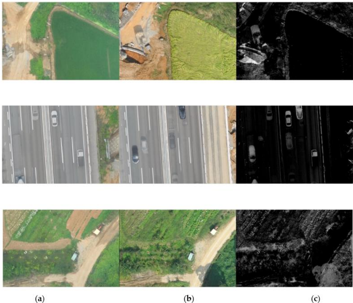
Figure 6. Results obtained using the image difference method; (a) and (b) display bitemporal images. (c) Result obtained using the image difference method.
