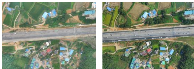
Figure 5. Orthoimages of some areas using (left) the first flight data and (right) third flight data.
