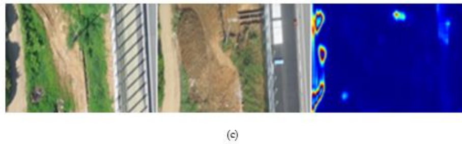
Figure 3. Cases of errors while detecting changes based on general change detection data: (a) Construction equipment, (b) automobile, (c) shadow. The left figures are time 1 images, the middle figures are time 2 images, and the right figures show the results obtained using change detection.
