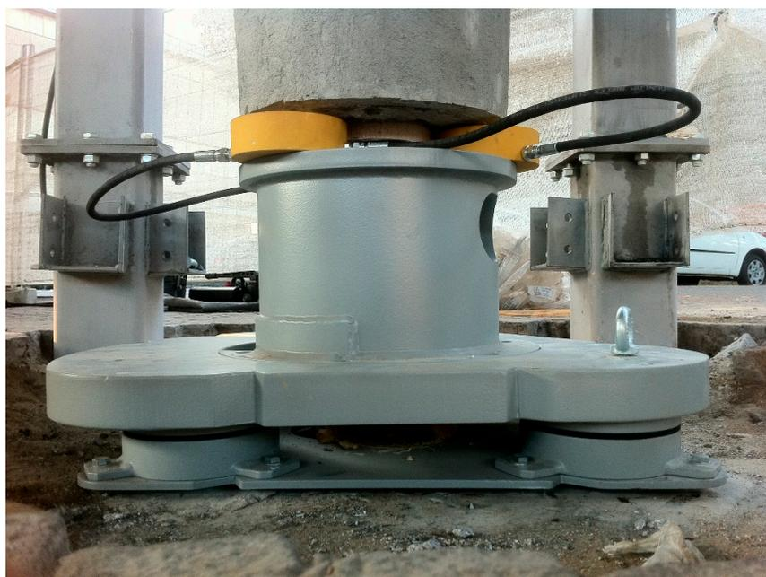
**Figure 19.** Picture of one of the tripods during its loading by means of three hydraulic jacks.
