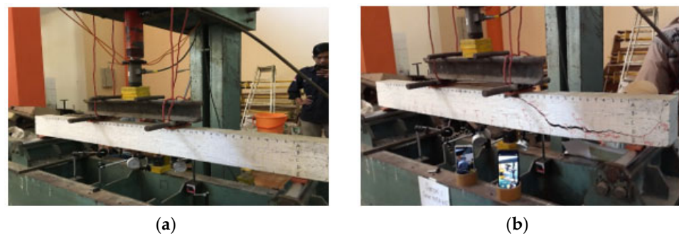
Figure 4. Testing the specimen beam (a) before and (b) after the beam shear failure.
