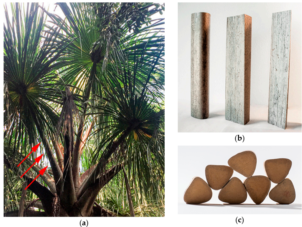
Figure 1. Buriti foam: (a) palm leaves with red arrows highlighting the petiole from which the vegetable foam is taken, (b) petiole longitudinal section, and (c) petiole cross-section.
