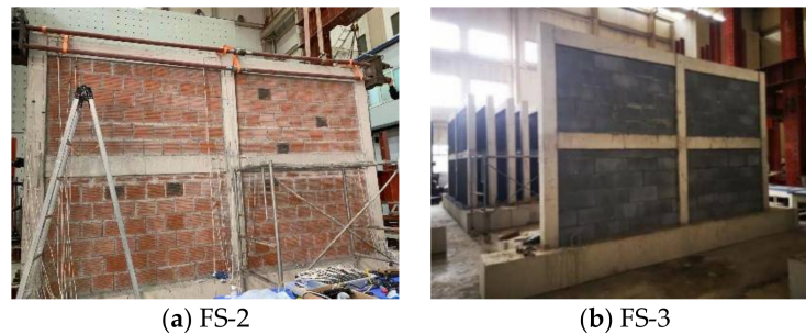
Figure 2. Specimens with infill walls.
