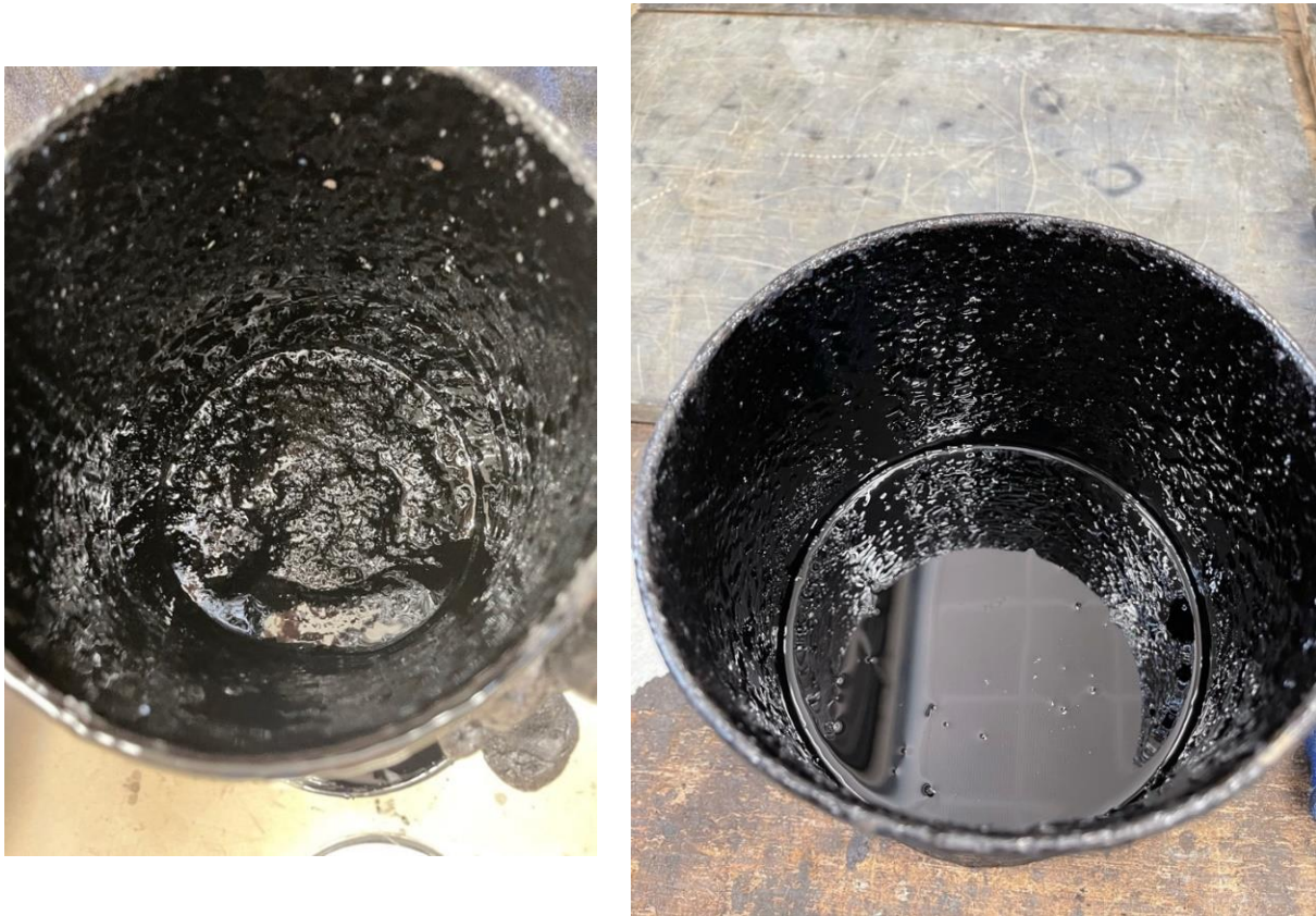
Figure 5. EPDM residue in bitumen.
