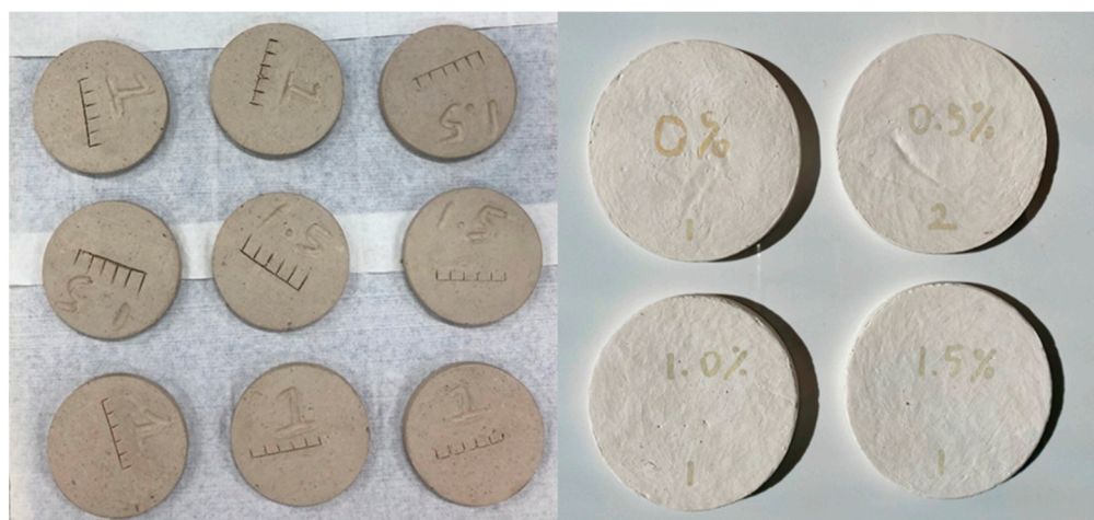
Figure 2. Pictures of ceramic tiles (left: freshly compacted; right: fired).
