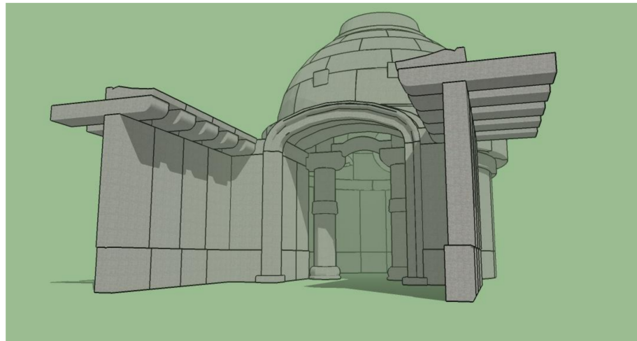
Figure 22. Model for the first structural study, assuming the absence of ‘forearms’.
