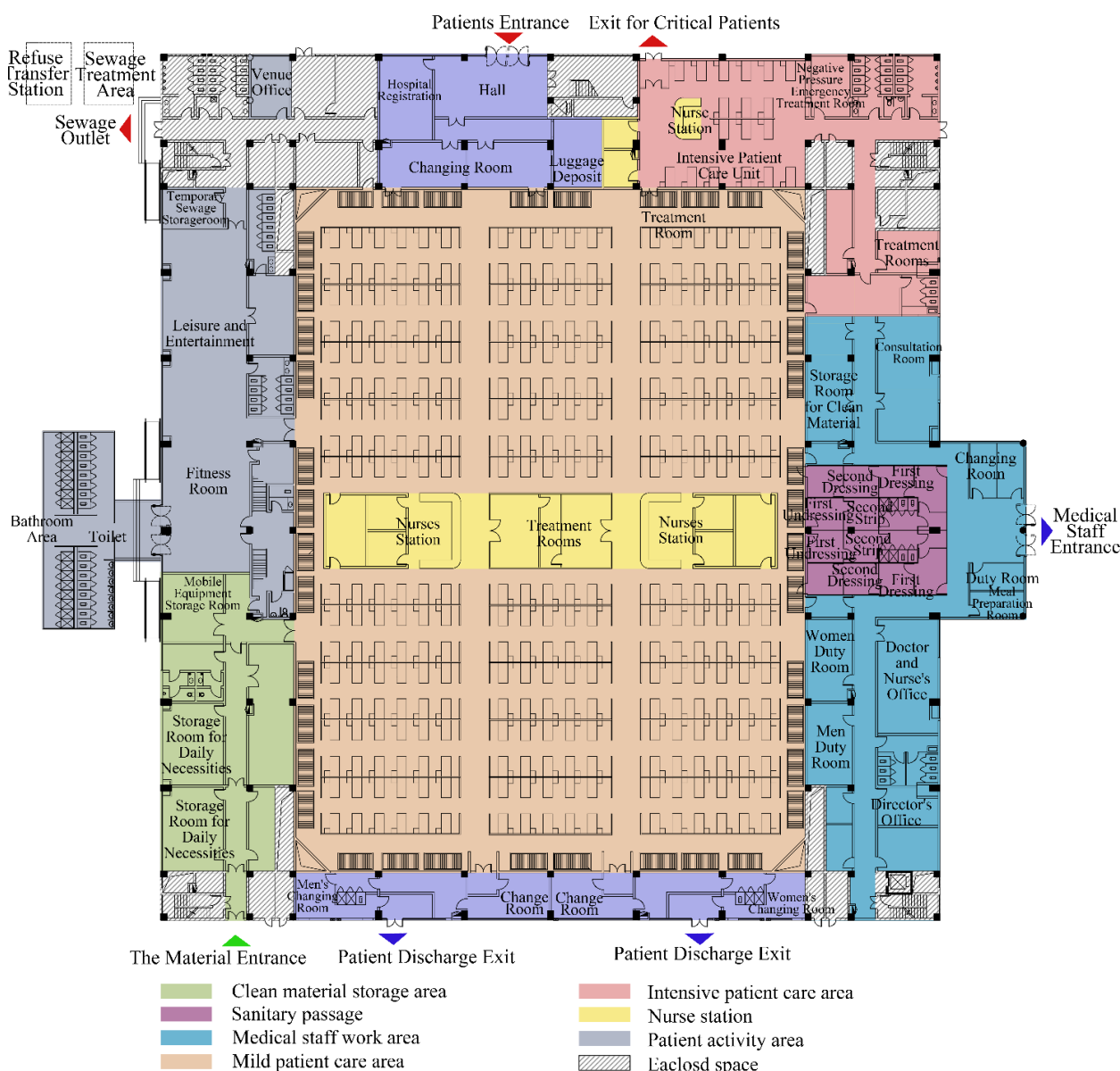
Figure 3. Fangcang shelter hospital renovated from a gymnasium of a university in Guangzhou by the authors.
