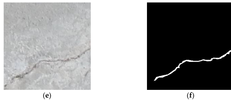
Figure 12. Original and manually labelled images. (a) Image I; (b) labelled image I; (c) image II; (d) labelled image II; (e) image III; (f) labelled image III.
