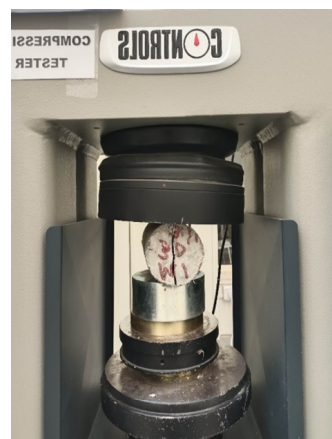
(e) Splitting tensile strength testing
