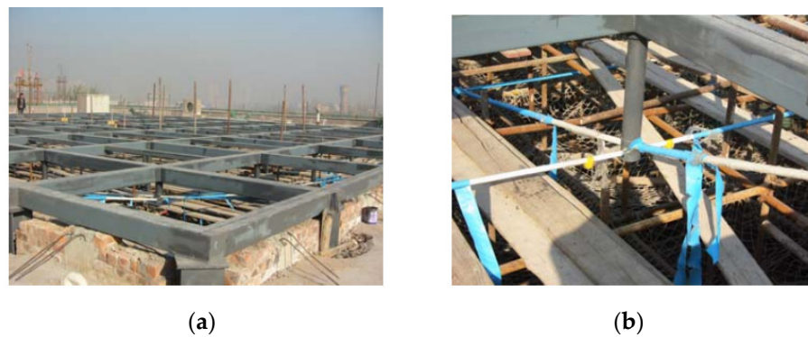
Figure 17. (a) Bidirectional string structure used in the experiment. (b) Frequency test of the bidirectional string structure.
