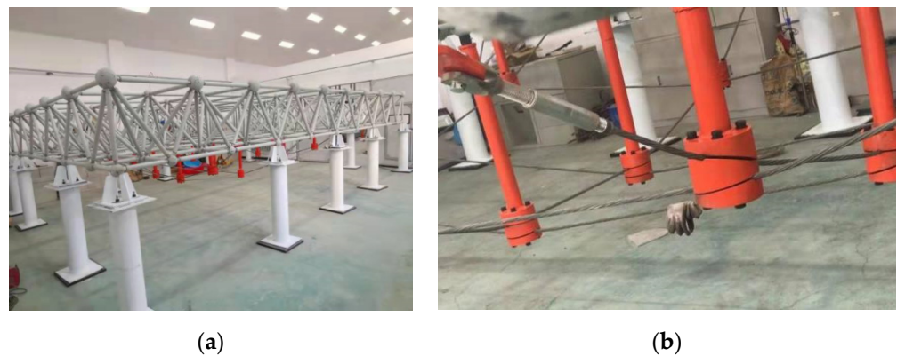
Figure 12. (a) Large-span space structure cable force identification test platform. (b) Cable laying.
