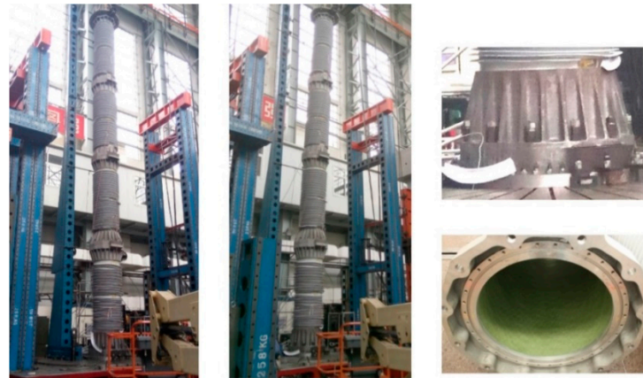
Figure 14. Cantilever bending test of composite insulators retrofitted by shear stiffeners and cast iron flange.
