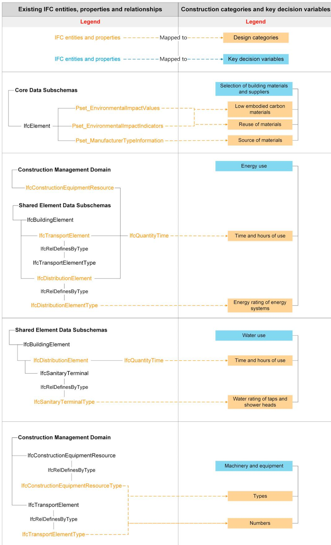
Figure 10. Existing IFC entities, properties, and relationships representing construction categories
