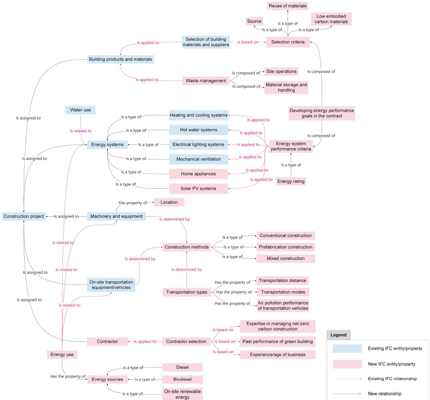
**Figure 14.** Illustration of an extension of additional entities, properties, and relationships to represent key decision variables affecting net-zero-carbon building outcomes at construction stage, and the links to the existing IFC entities.
