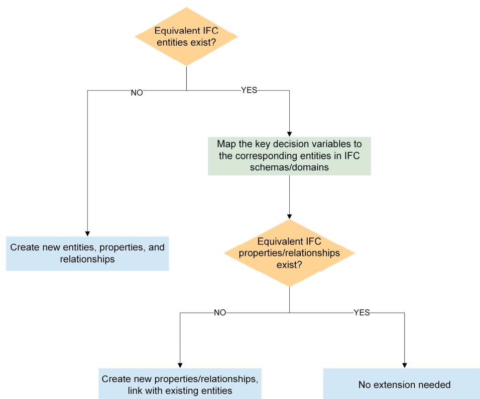
**Figure 3.** Mapping the identified key decision variables with the existing BIM/IFC schema.
