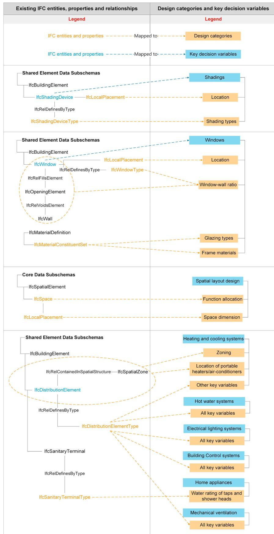
**Figure 9.** Existing IFC entities, properties, and relationships representing design categories and key decision variables affecting net-zero-carbon building outcomes at design stage (continued).
