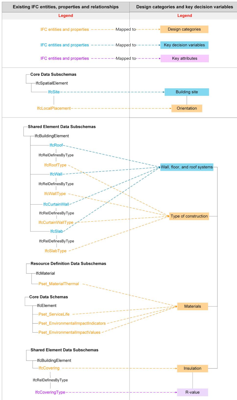
**Figure 8.** Existing IFC entities, properties, and relationships representing design categories and key decision variables affecting net-zero-carbon building outcomes at design stage.
