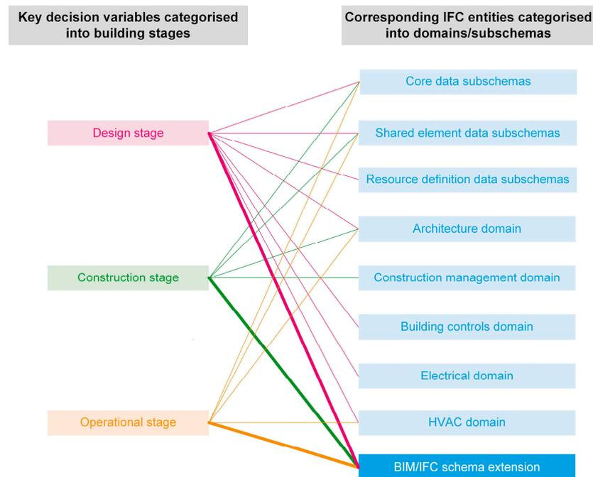
**Figure 7.** An outline of mapping results between the categories of key decision variables and subschemas and domains in BIM/IFC.
