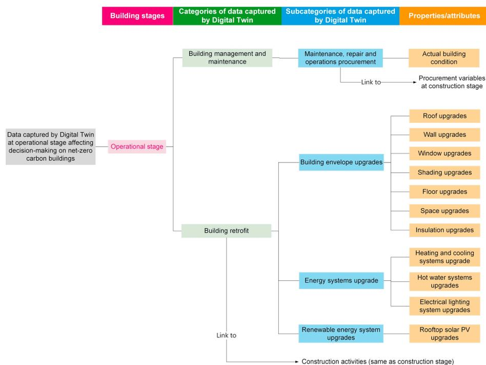
**Figure 18.** Data captured by DT at operational stage which affect decision-making for net-zero-carbon building.
