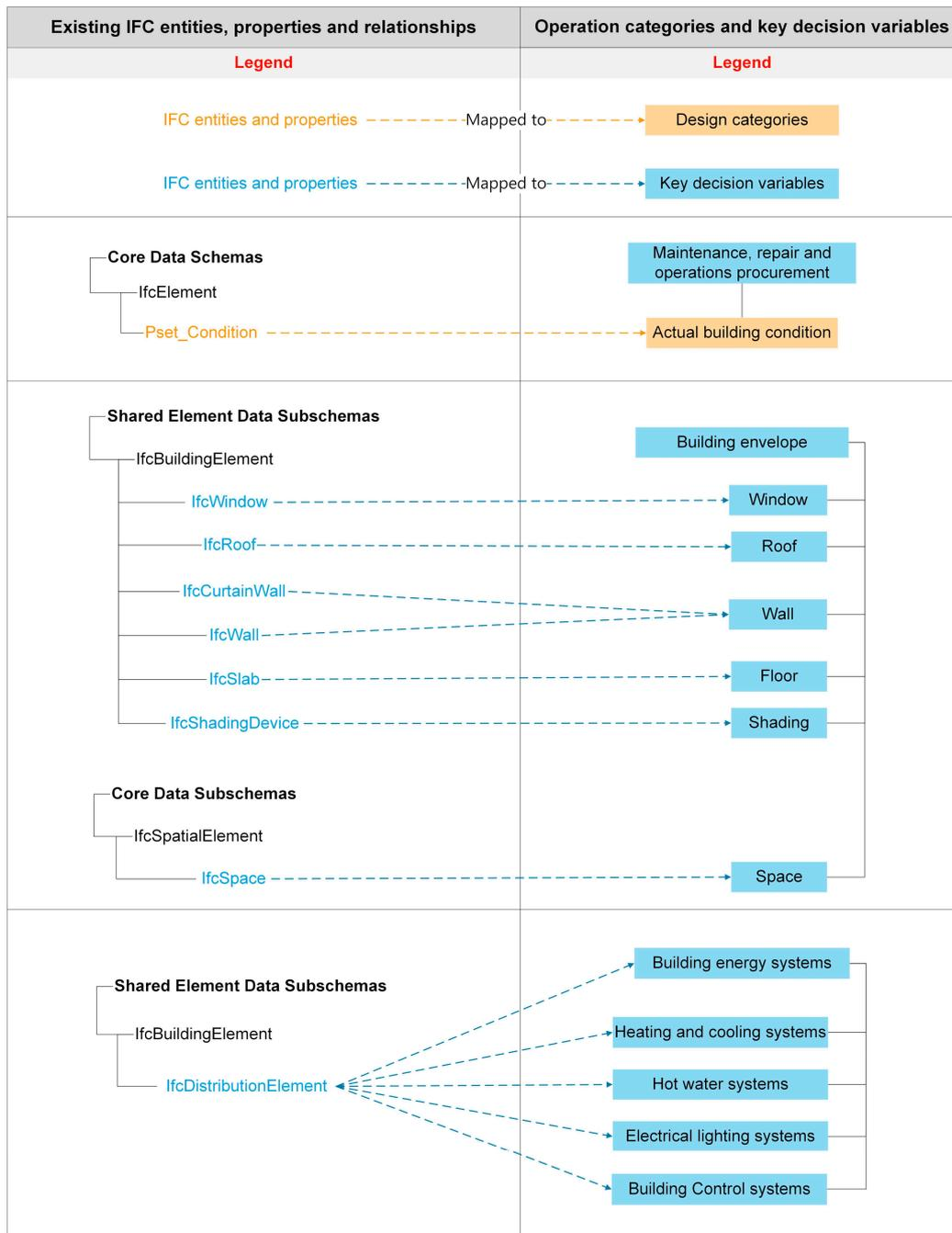
**Figure 11.** Existing IFC entities, properties, and relationships representing design categories and key decision variables affecting net-zero-carbon building outcomes at operational stage.
