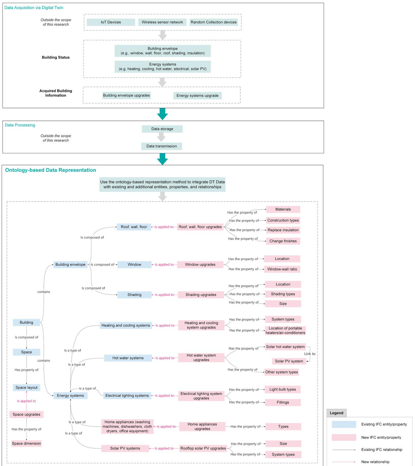
**Figure 19.** Illustration of DT data integrated into extension using the ontology-based representation method to represent key decision variables at operational stage.
