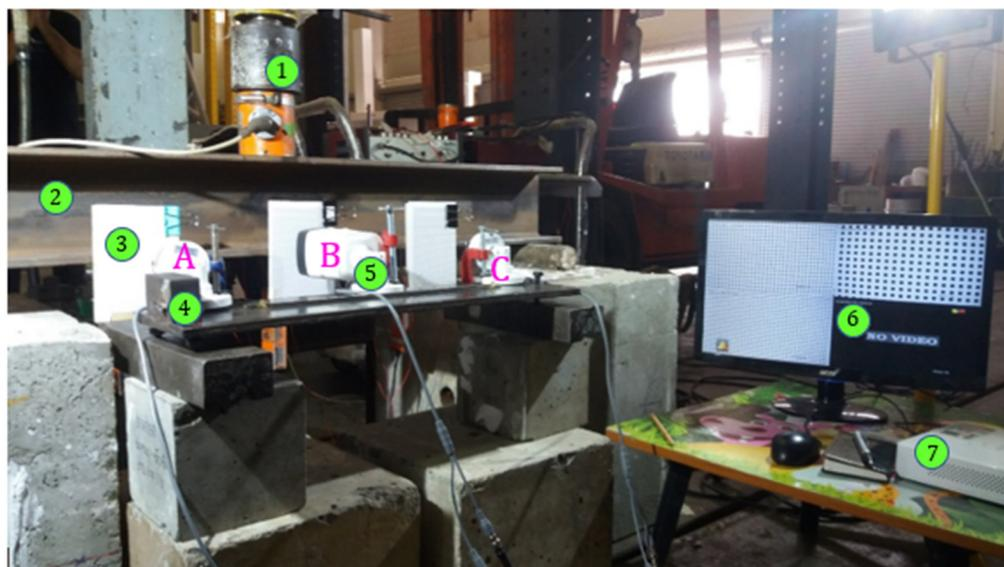
**Figure 7.** Photograph of the experimental setup in a specimen with labels. (1) Loading cell, (2) I-beam specimen, (3) grating panel, (4) linear guide (5) CCTV camera, (6) monitor for operating the camera, (7) DVR box, (A–C) camera positions.
