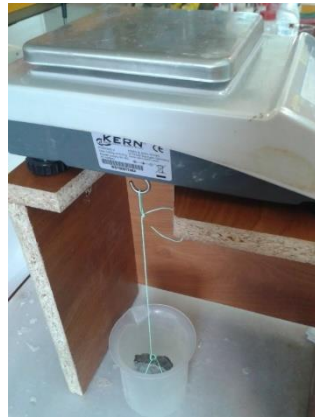
Figure 3. Apparatus for the immersed apparent mass determination.
