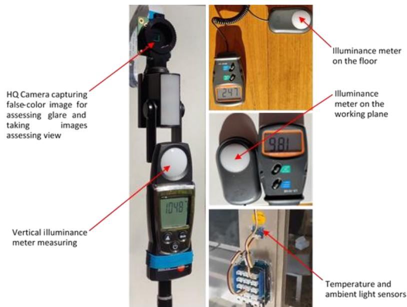
Figure 10. Field experiment validation of the simulation results.
