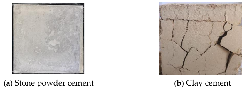
Figure 11. Destruction images of hardened bodies in natural state.
