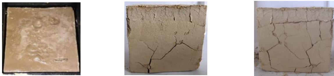
(a) Normal contraction stage (b) Residual shrinkage stage (c) Micro expansion stage
