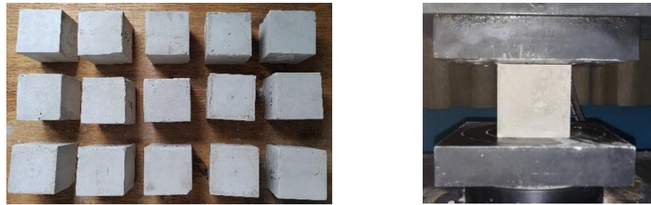
Figure 2. Standard stone powder hardened body specimens and compressive strength test.
