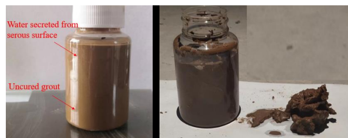
Figure 4. Clay cement slurry does not solidify after standing for half a year.
