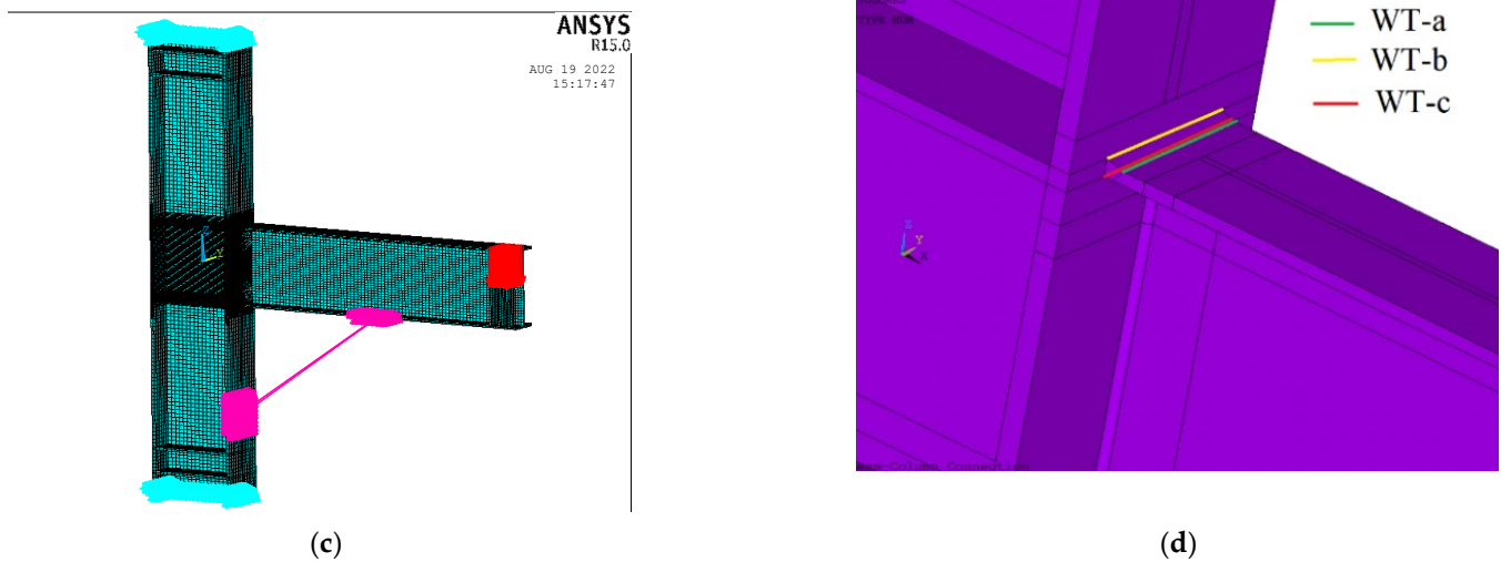
Figure 2. Finite element model of the connection. (a) Connection without the VFD. (b) Local view of the weld detail. (c) Connection with the VFD. (d) Definition of weld toe lines.
