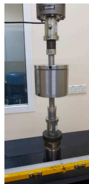
Figure 7. Product testing, showing force–displacement test and results for product under cyclical compression.
