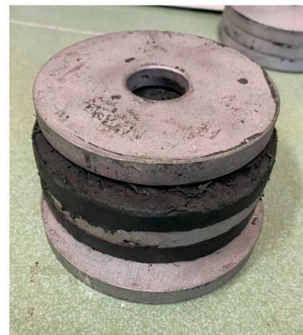
Figure 4. Typical isometric view and dimension of the proposed scaled-down hyperelastic composite damper.
