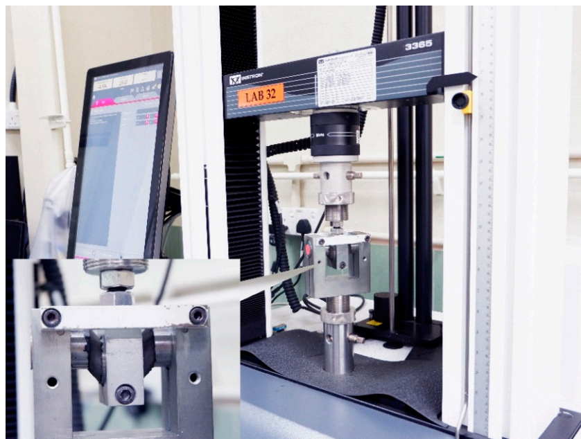
Figure 2. Double-shear testing using INSTRON servo-hydraulic testing machine.
