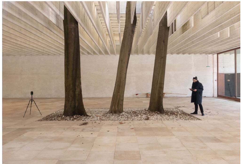
Figure 4. Case study step 1. Three-dimensional scanning the pavilion site. Source: Author.
