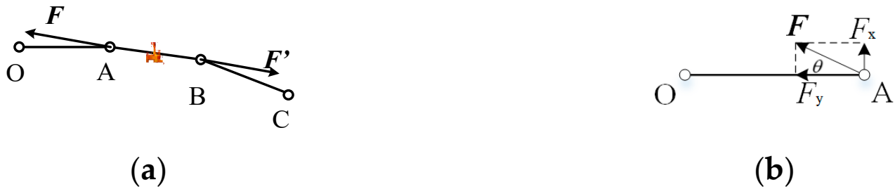
Figure 11. Schematic diagram of radial member force. (a) Unbalanced force diagram; (b) decomposition of force.
