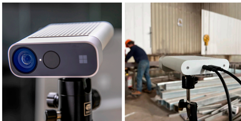
Figure 7. Microsoft Azure Kinect for data collection in a steel modular construction factory.
