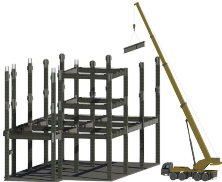
Figure 11. Building construction drawing.
