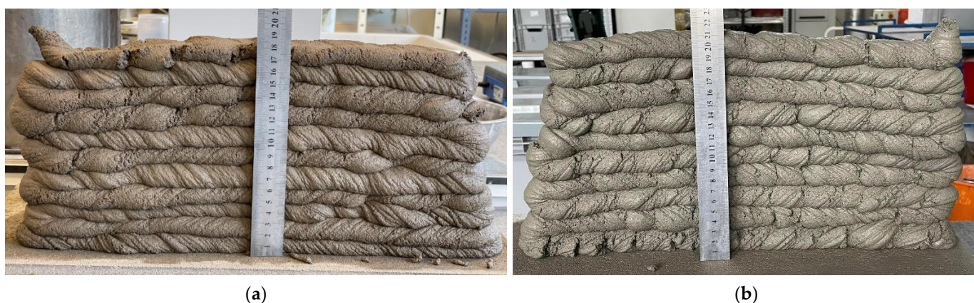
Figure 10. Examples of mixtures that have not collapsed before reaching demanded number of layers and thus succeeded to meet the requirements of the test (a) mixture SAP_35HFA, (b) mixture SAP.
