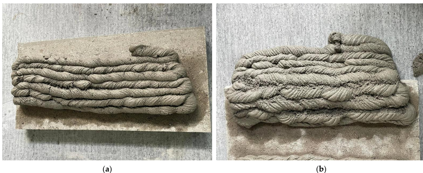
Figure 9. Examples of mixtures that have collapsed before reaching demanded number of layers and thus failed to meet the requirements of the test (a) mixture C_A, (b) mixture C_B.
