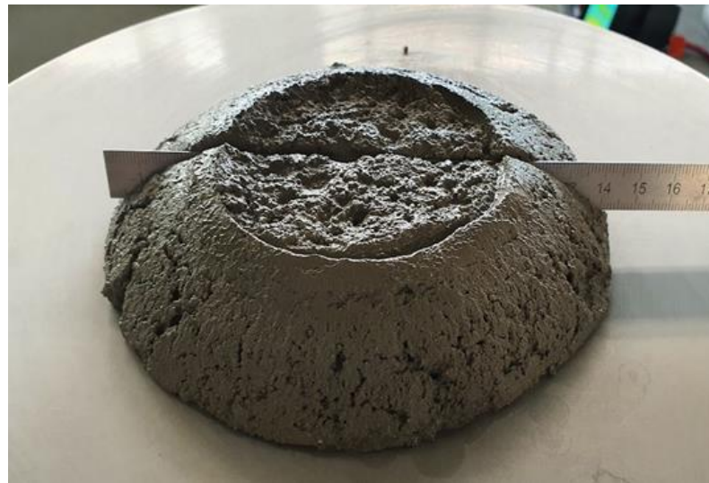
Figure 11. Consistency of fresh mortar with printable consistency.
