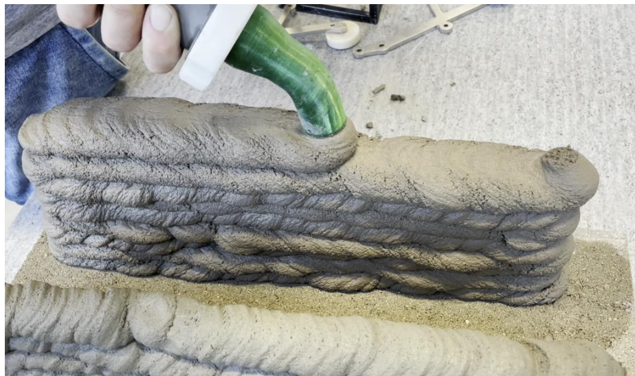
Figure 8. The process of extruding a line onto a solid, moistened surface.
