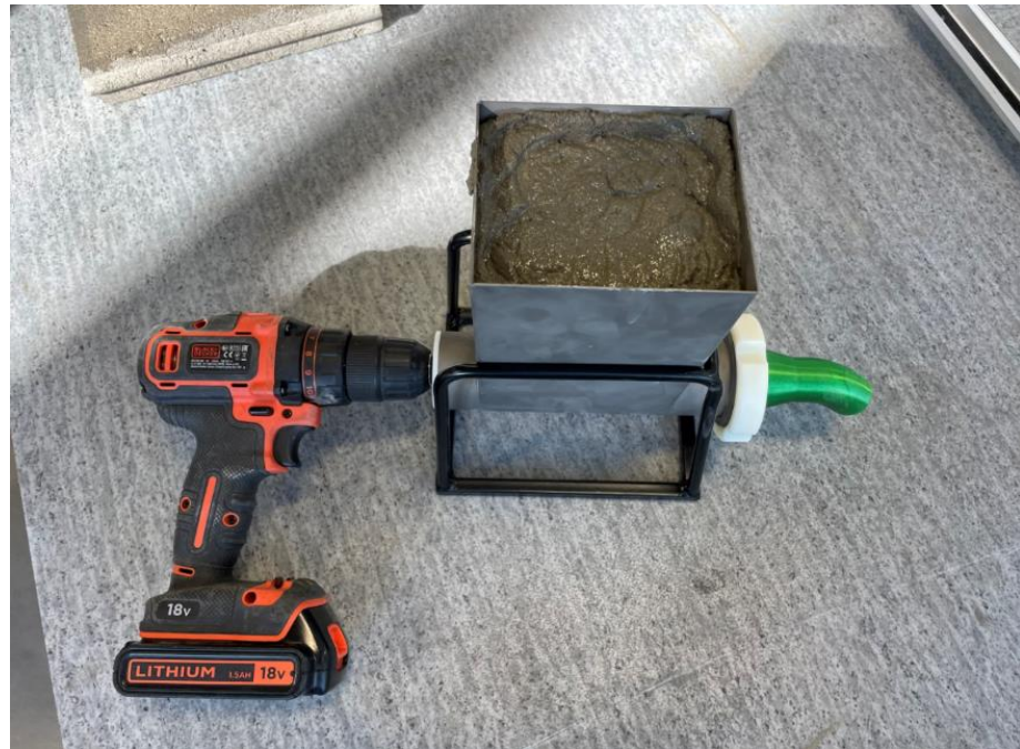
Figure 7. Filled in extrusion equipment with attached power drill.
